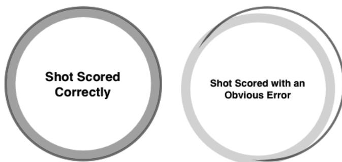
On rare occasions, a badly torn or irregular shot hole will cause the VIS scoring system to misread the shot hole location. The diagram depicts a shot hole that is scored correctly with the VIS system and a shot hole with an obvious error. As a guiding principle, if the VIS system scoring ring is more than two scoring ring widths away from the apparent shot hole, the Statistical Officer may rule that this is an obvious error and make a manual correction to the scoring ring location and score.
